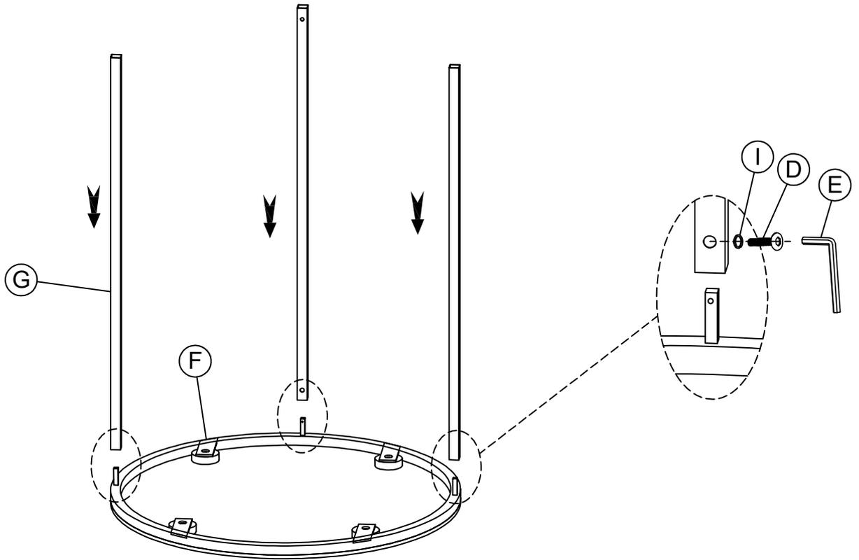
Step 4: Using the Allen key to tighten all bolts.
